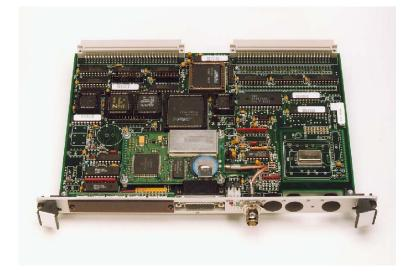
The VME-SyncClock32 from Brandywine Communications provides precision time with zero latency to the host computer over the VME bus. An on-board microprocessor automatically synchronizes the clock to reference signal inputs. The reference signal inputs can be 1 PPS, IRIG A or B and NASA 36 time codes. GPS and Have Quick inputs are optionally available. The clock can free run and be set by commands from the host over the VME bus.
